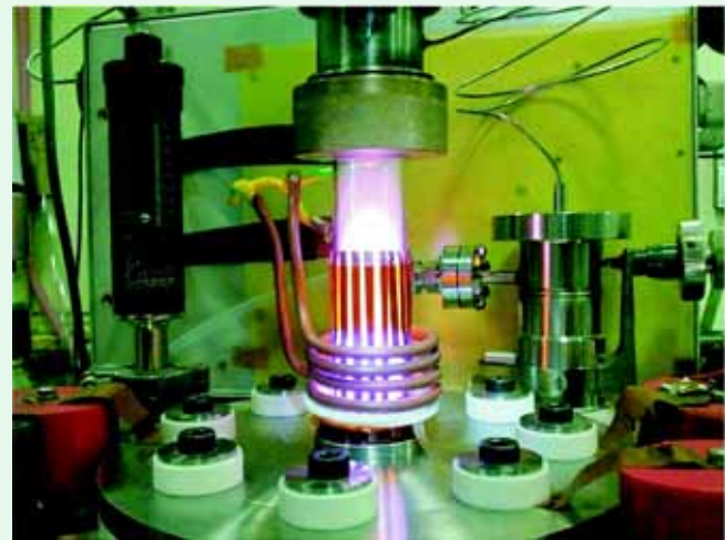
Fig 1 RF ion source with Argon plasma
