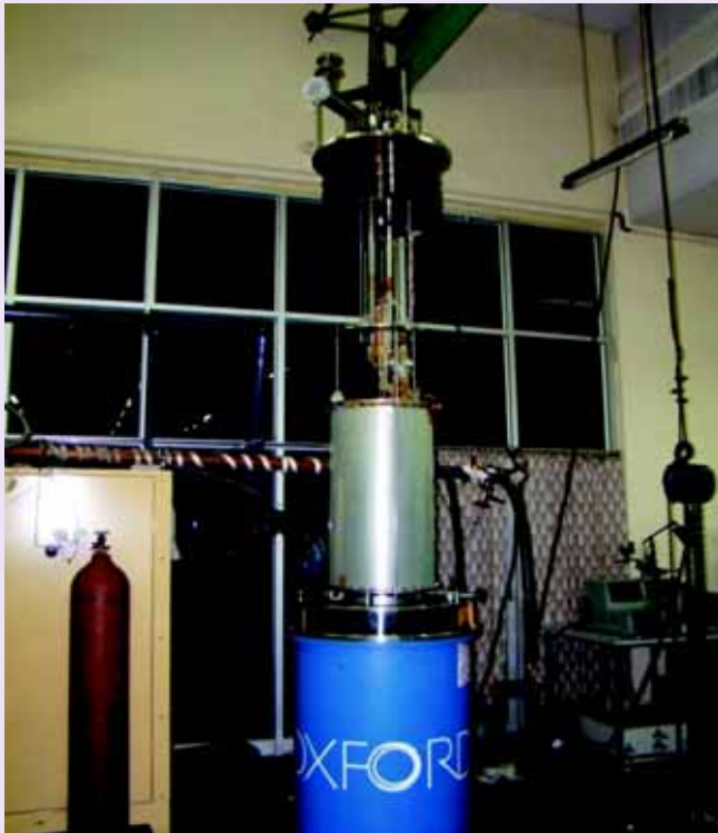
Fig 2 Prototype SMES coil during assembly in cryostat
