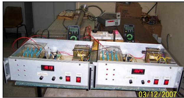
High voltage power converter
