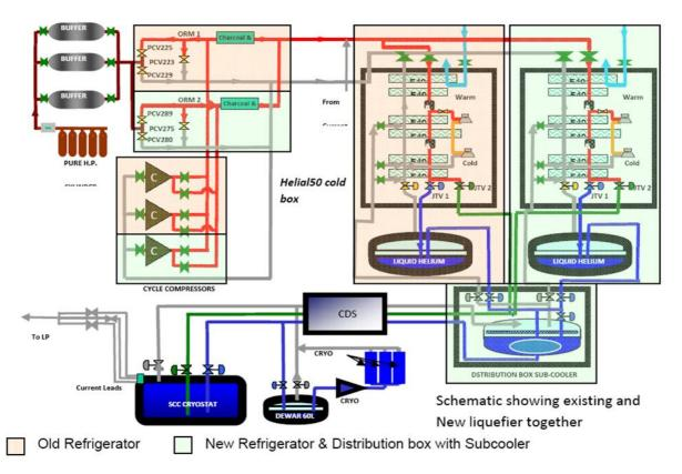
Figure 1 Schematic View of the total cryogenic system of VECC
