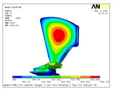
Fig. 4: Temperature distribution in Trimmer Rotor assembly of VEC Cyclotron
