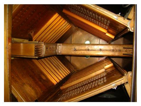
Fig.1: RF Resonator Cavity of VEC Cyclotron
