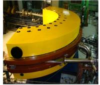
Fig. 2: Analysing magnet with SS beam chamber
