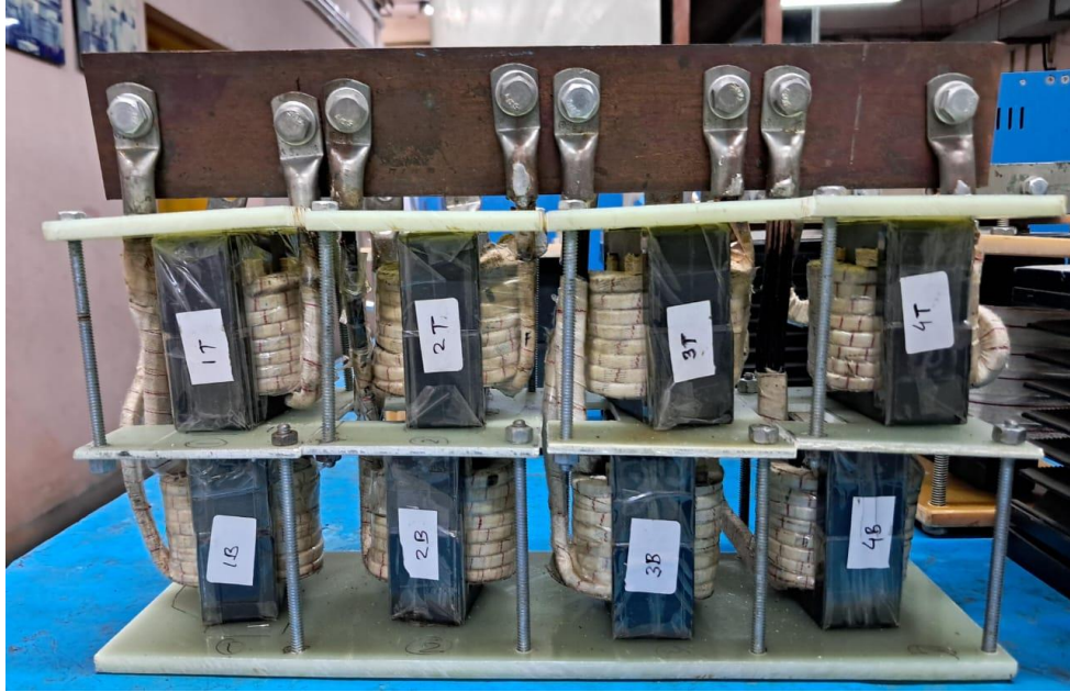
Fig 1 a: Clockwise from top left, Steering Magnet Coil for K130 RTC, 125 VA Transformer for BRIT, Set of 8 ferrite core inductors for Power Supply applications
