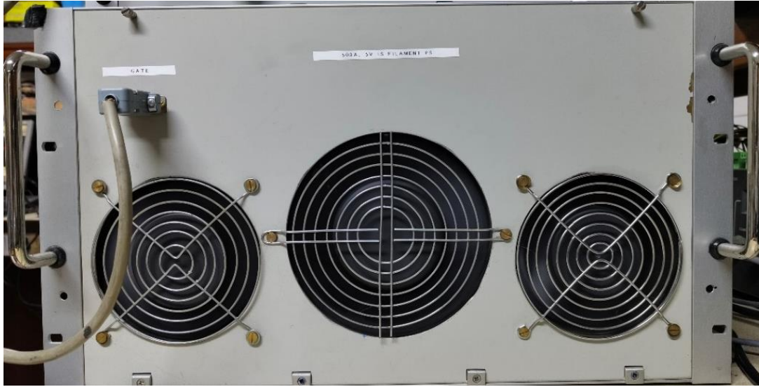
Filament Power Supply Power Cabinet
