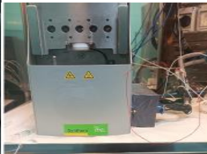
Figure (counter clockwise from top): The program sequences are on the laptop screen (GUI), BVSynth Controller unit, Retrofitted Synthera for BVSynth interfacing
