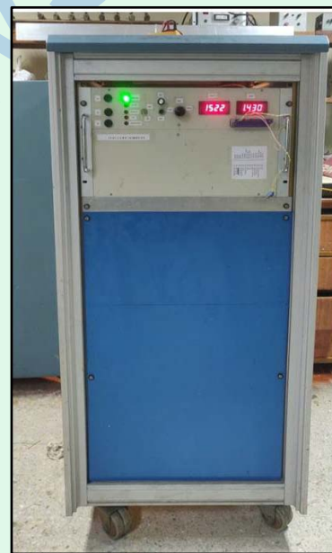
Figure 3: Final assembled power supply inside rack
