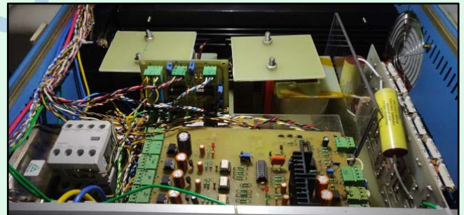
Figure 3: Internal view of puller power supply
