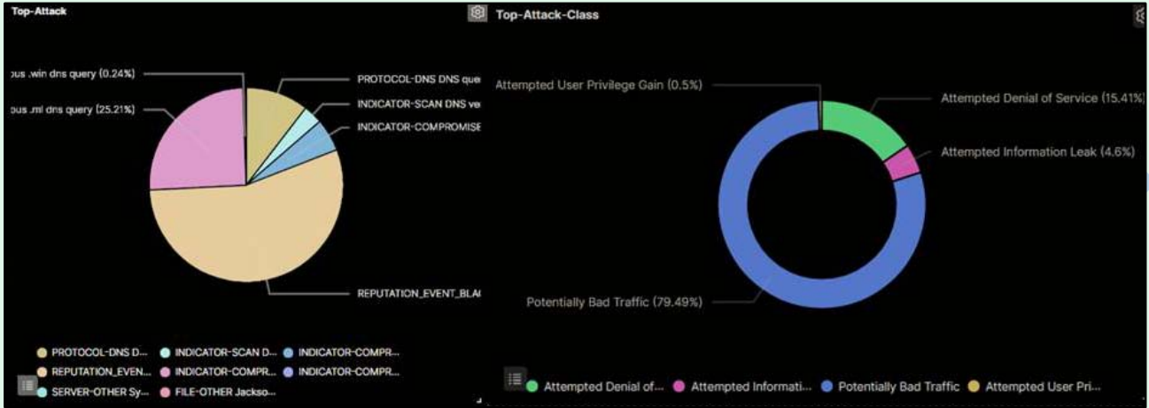
Figure 1: Top Attacks and Top Attack Classes as detected by SNORT are graphically displayed in ELK dashboard.
