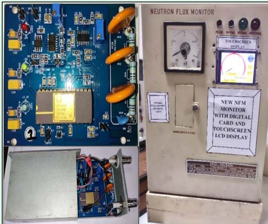
CSPC module with 28 Pin DIP VECC003 ASIC and NFM monitor with touch-panel display
