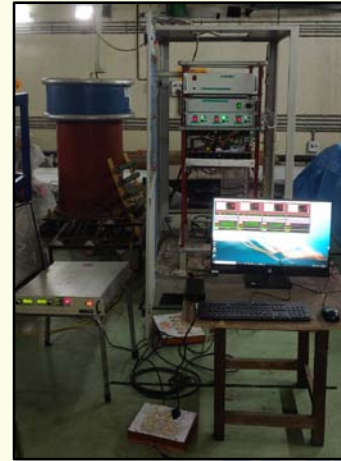
Figure 3 Power supplies during testing on dummy load
