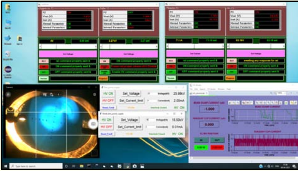
Figure 2 Screenshot of control PC during beam tuning showing beam and GUI of supervisory systems for power supply and beam monitoring
