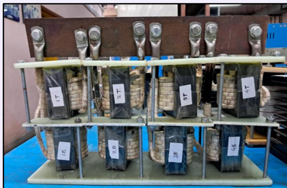
Figure 2: Set of 8 ferrite core inductors for Power Supply applications
