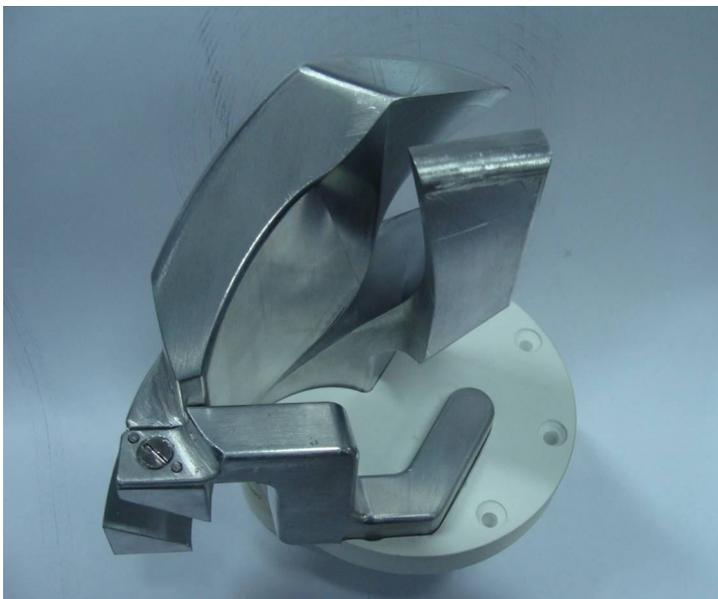
Fig. 5: Spiral inflector for high current ion source
