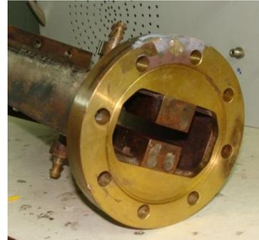
Fig. 4: Water cooled ridged wave guide
