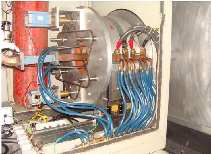
Fig. 1: High Current Ion Source Assembly
