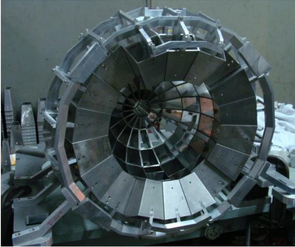
Fig. 2. Final assembly of the backward part of CPDA
