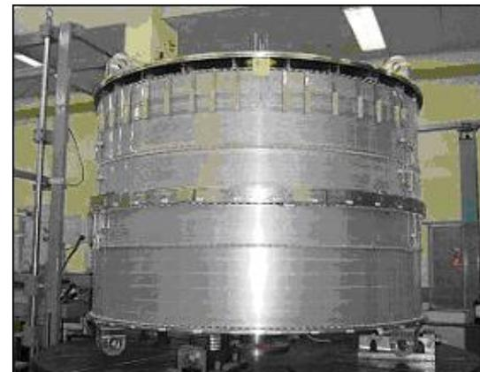
*Completed K-500 Superconducting Coil*
