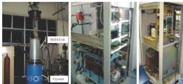
Figure 2: (from left) a). SMES coil, b). DC-DC chopper, c). VSI
