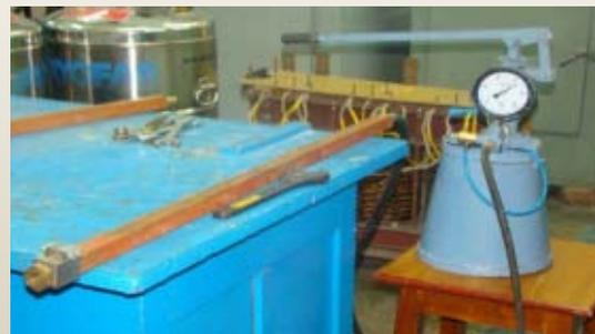
Figure 4: Hydraulic Test bench for joint leak-testing at 13.5 bar.
