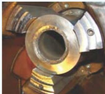
**Figure 4:** Central Plug with the modified hill addition
