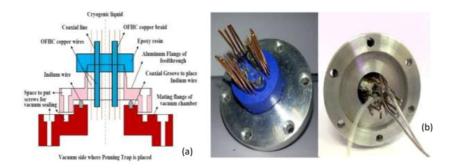
FIG. 1. (a) A schematic drawing of the feedthrough and the mating angle of the vacuum chamber (not drawn to scale)
