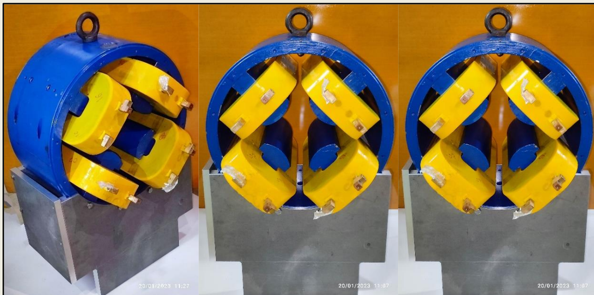
Figure 2: Picture of quadrupole magnet after assembly
