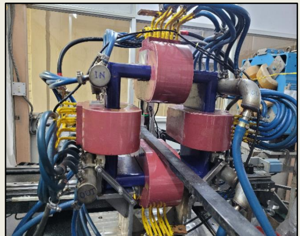
Figure 4: Final assembly of steering magnet with water line.
