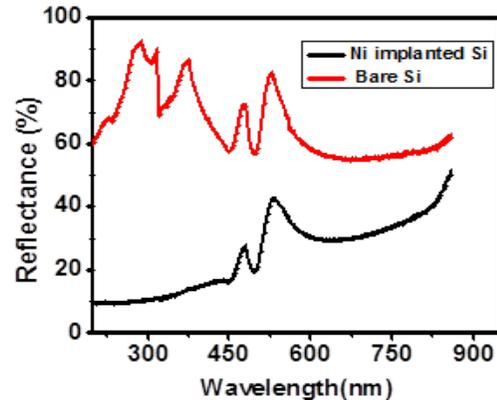
Reflectance data showing the huge absorption of light by nanopatterned and Ni<sub>2</sub>Si embedded a-Si compared to bare Si.
