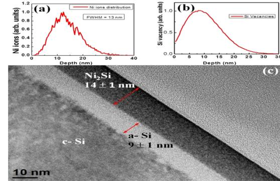
(a) implanted Ni atoms and, (b) Si vacancy due to 10 keV Ni<sup>+</sup> ion bombardment on Si at normal incidence; (c) Cross-sectional TEM view of 10 keV Ni<sup>+</sup> ion implanted Si(100).
