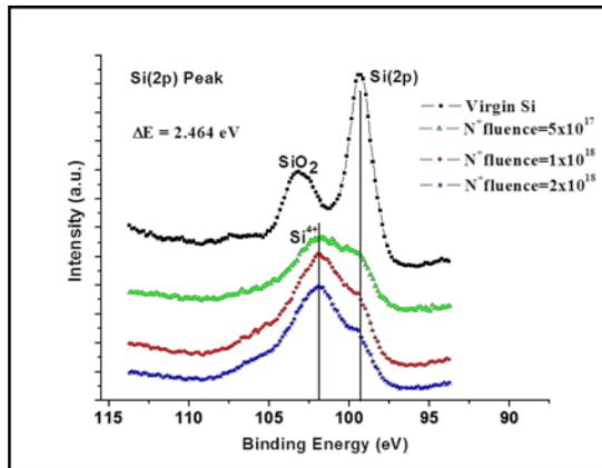
X ray photoelectron spectroscopy data showing the shift of Si(2p) peak towards the higher binding energy for  $N^+$  ion implanted rippled Si surfaces at ion fluences  $5 \times 10^{17}$ ,  $1 \times 10^{18}$  and  $2 \times 10^{18}$  ions/cm<sup>2</sup> compared to virgin Si surface. The shifted does not change with ion fluence but peak intensity decreases with Nitrogen fluence. The change of oxidation state of Si due to Nitrogen implantation indicates the Silicon Nitride formation.
