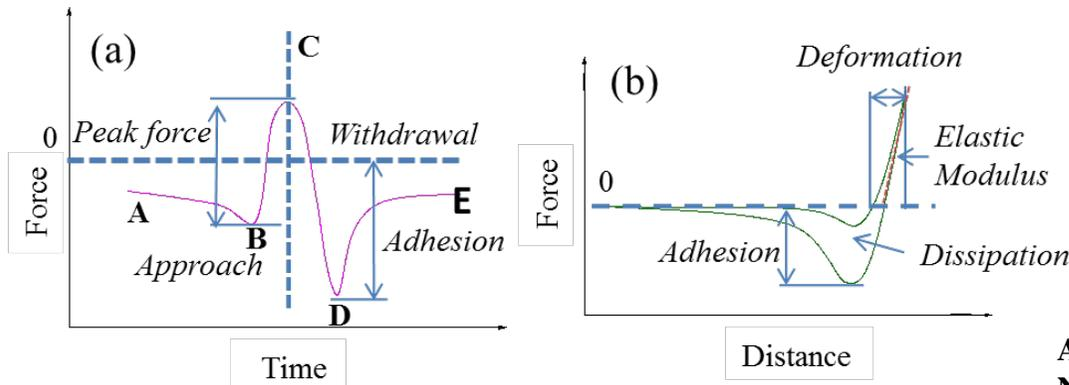
(a) Force-time representation, showing the principle of peak force operation of the AFM. (b) showing different peak force channels.
