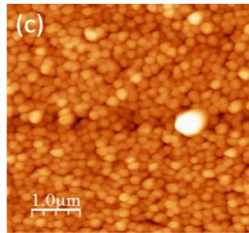
Ag nanoparticles on O<sup>+</sup> ion bombarded Ge substrate
