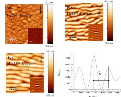
AFM image showing the topography of the irradiated sample with  $N^+$  ions at a fluence of (a)  $5 \times 10^{17}$  ions/cm<sup>2</sup>, (b)  $1 \times 10^{18}$  ions/cm<sup>2</sup> and (c)  $2 \times 10^{18}$  ions/cm<sup>2</sup>. (d) Shows the 1D-autocorrelation function along the wave vector of the ripple structure
