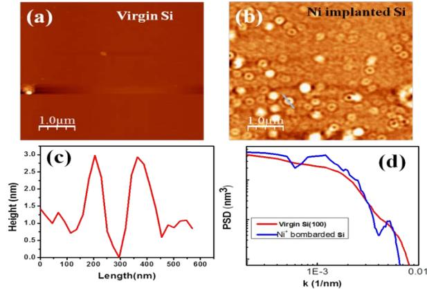
AFM topography of (a) Virgin Si(100) surface, (b) 10 keV Ni<sup>+</sup> (fluence  $1 \times 10^{17}$ ) ion implanted Si(100) surface showing rim surrounded crater structure, (c) line profile along the marked line on (b), (d) The Power Spectral Density profiles of the virgin and the irradiated Si.
