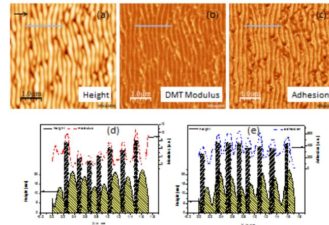
Peak force QNM data of the irradiated samples at a fluence of  $2 \times 10^{18}$  ions/cm<sup>2</sup>. Images of (a) height, (b) elastic modulus and (c) adhesion of the nitrogen ion induced rippled surface. (d) and (e) shows the height (in lower panel) with modulus (in upper panel) and height (in lower panel) with adhesion (in upper panel) profile respectively along the line on (a), (b) and (c). Periodic variations of modulus and adhesion are clearly observed.
