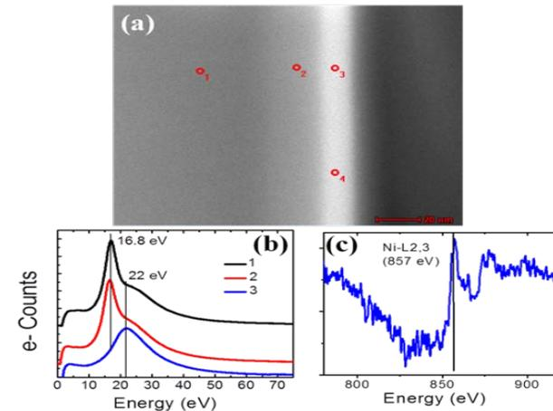
Cross-sectional STEM-HAADF and EELS spectra showing Nickel silicide formation during 10 keV Ni<sup>+</sup> ion bombardment on Si (a) Cross sectional STEM-HAADF image for ion fluence of  $1 \times 10^{17}$  ions/cm<sup>2</sup>, (b) Low-loss spectra at t positions 1, 2, 3 of (a), (c) Core-loss spectra at Ni-L<sub>2,3</sub>-edge at position 4 of (a).
