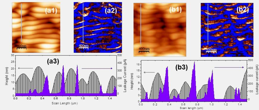
Ripple topography on thin ZnO films by grazing and oblique incidence ion sputtering, *Appl. Surf. Sci.* 257, 6775 (2011)
