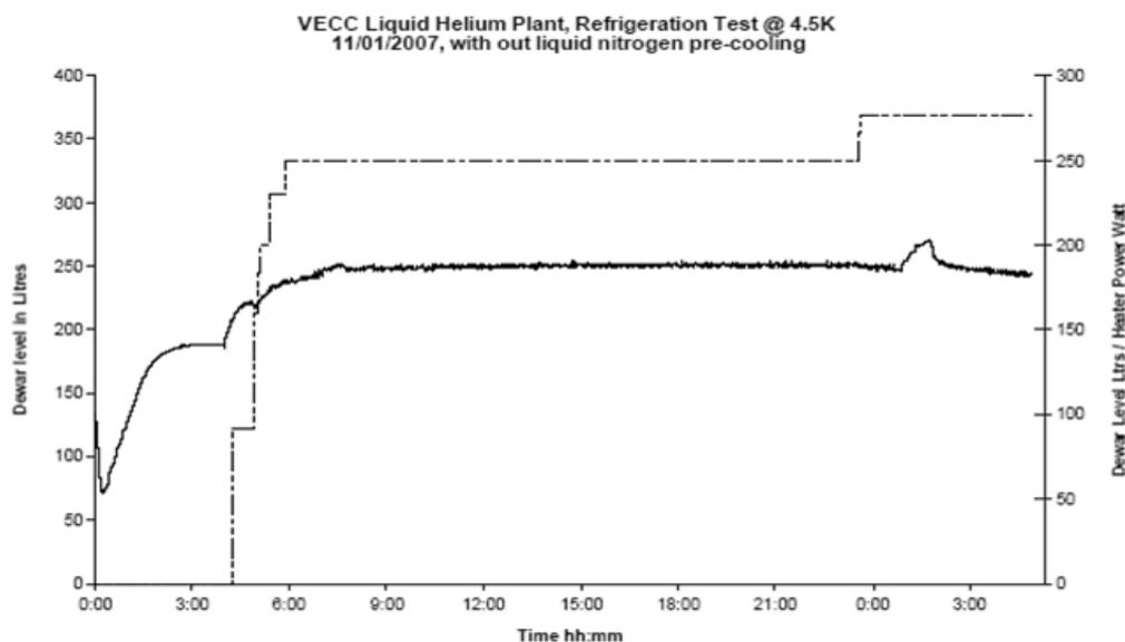
Figure 7- Test Result of First Helium Liquefier
