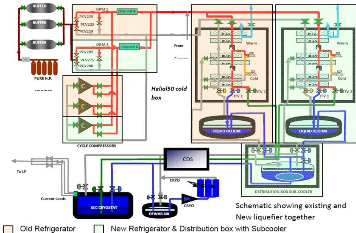
Figure 1 Schematic View of the total cryogenic system of VECC
