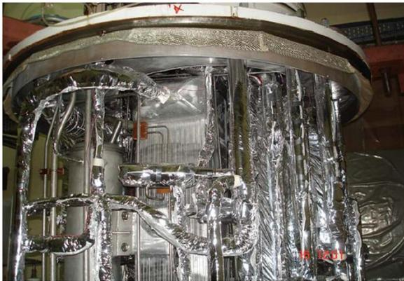
Figure 2: Internal view of the cold box of Helium Refrigerator 1
