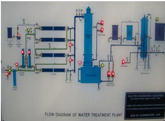
Fig. 3: RO plant mimic diagram
