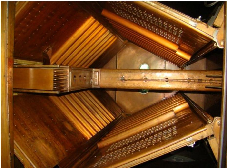
Fig.1: RF Resonator Cavity of VEC Cyclotron
