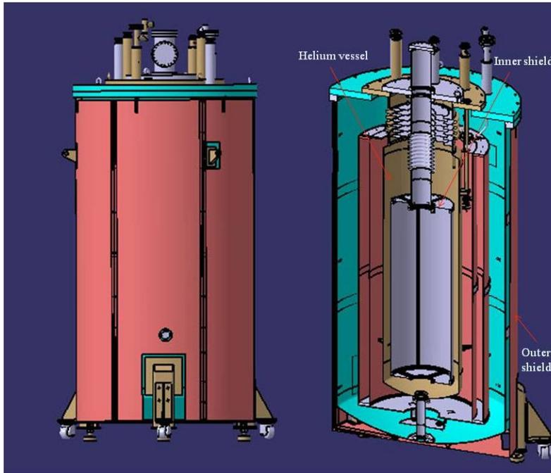
Model of test cryostat
