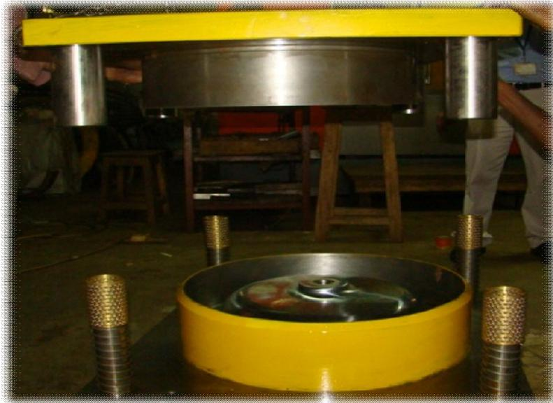
Figure C: Die-Punch for deep drawing trial
