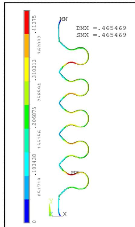
Figure B: Deformation due to cooldown and
